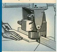
MOLDING . . . the molding head gives the Sawsmith unlimited versatility for shaping. Tilting of the spindle affords additional shapes from any set of cutter knives!
