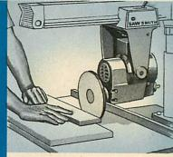
SANDING . . . using disc or drum sanders, the spindle and table can be adjusted, the spindle speed varied. Sawsmith gives fast, efficient sanding of any surface!
