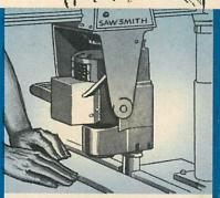
JOINTING . . . by using a jointer head (has 21/2" capacity), the Sawsmith quickly and easily produces an exacting, perfectly smooth surface for jointing!
